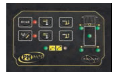
Remote controlled outriggers and MCS system
